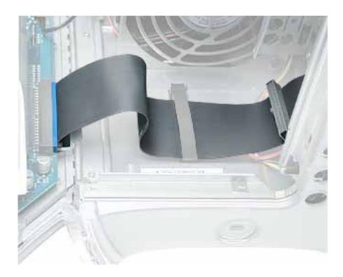
2. **Note:** To reach the ATA cable connector on the back hard drive, you may need to remove the carrier. If so, use a Phillips screwdriver to remove the mounting screw that holds the carrier to the chassis. Then pull the carrier lever forward and slide up the carrier to disconnect it from the chassis. **(Figure 3)**
